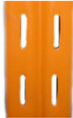
**MULTIRACK** columns consist of cold formed perforated ribbed & lipped c-channels to provide an extremely high axial load capacity and maximum tensional & buckling resistance. The perforated slits are minimal in size unlike any other 'key-hole' type or similar systems, which require large holes detrimental to the structural strength of the column.
