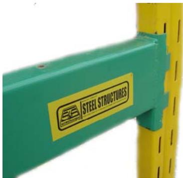
**MULTIRACK** beams comprise double cold formed channels compounded to form a hollow section with inserted stiffeners, designed to carry heavy loads with minimal twist. Various beam sizes are available to suit varying load requirements.
